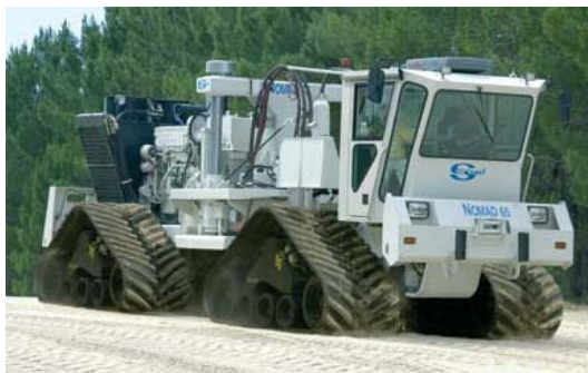
Off-road seismic vibrator Nomad 65T
